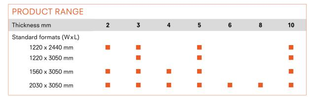
The given measurements are standard dimensions, ex works. Special sheet sizes upon request, sheets cut to size can be obtained from your distributor.
